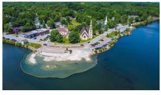
A living shoreline provides protection from flooding, erosion, and storm surge through nature-based infrastructure as opposed to the hard rock armouring typically seen along Nova Scotia coastlines. This innovative project will also filter stormwater runoff, stabilize the shoreline bank, reduce wave energy, and enhance coastal habitat. We hope this pilot project will assist in securing support to complete the Living Shoreline all along Edgewater Street.
