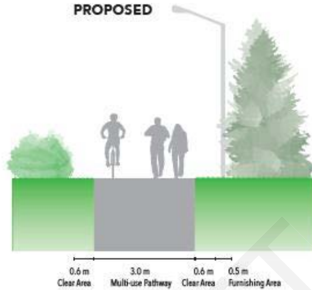
Figure 10: Proposed Pathway Cross-section
