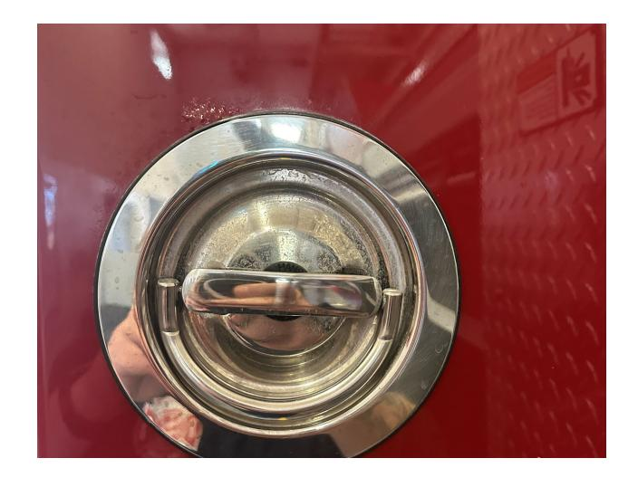
Surface corrosion around slam door handle.
