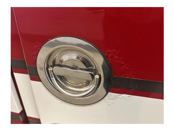
Light corrosion around slam door handle
