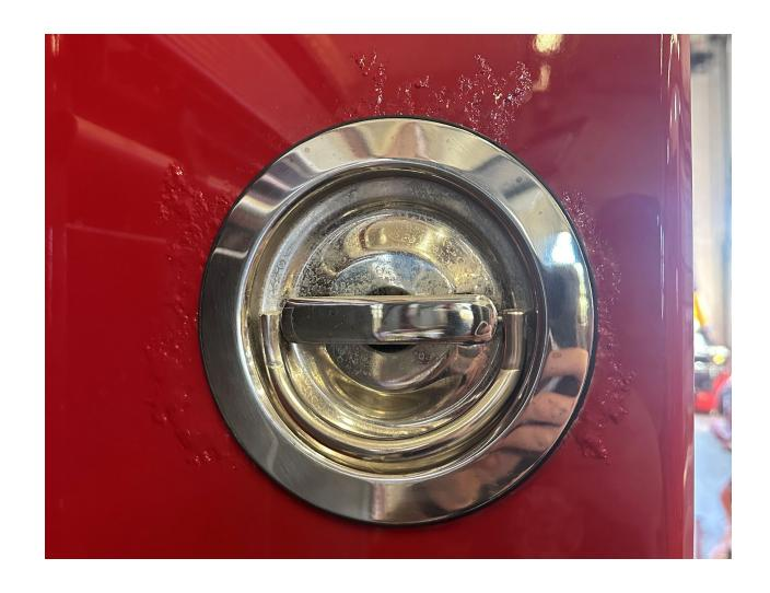
Surface corrosion around slam door handle
