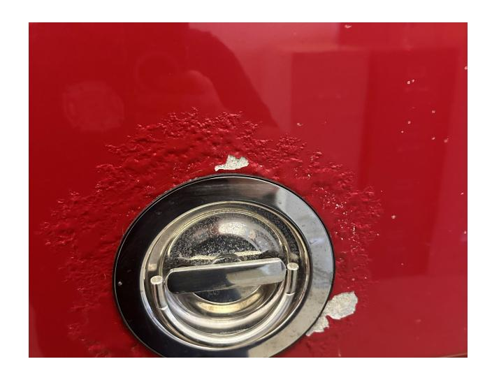
Light corrosion around slam door handle.
